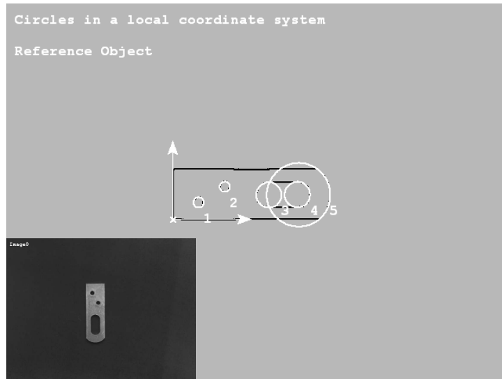
Figure 5.2: Circles fitted to the rotated contours of the reference image.
