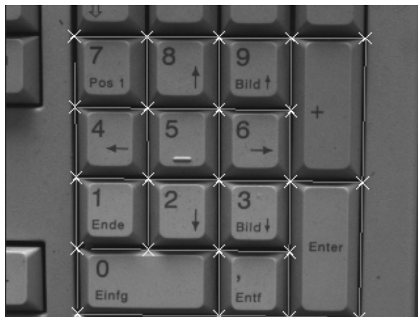
Figure 4.11: Lines and junction points representing the grid that separates the keys.
