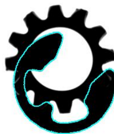
Figure 1.7: Occlusions can be handled by shape-based matching.
