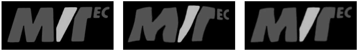
Figure 3.21: From left to right: template image, corresponding part of the search image, rectified image.
