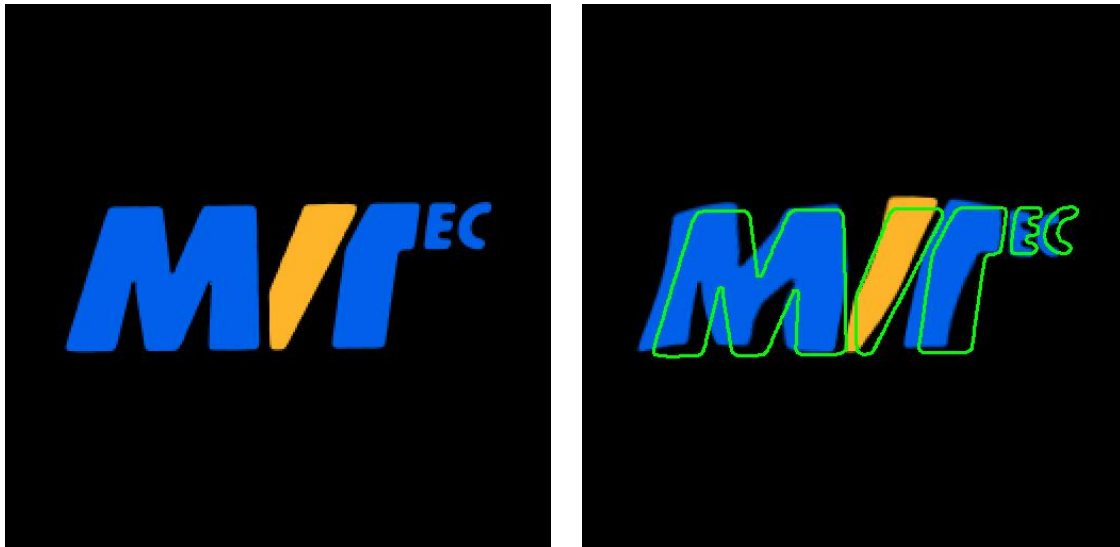
Figure 3.20: (left) “MVTec” logo used for the model creation; (right) deformed logo instance overlaid by the model contours.
