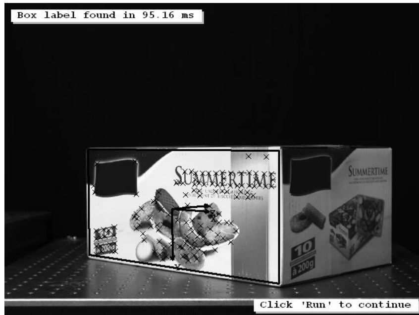
Figure 3.30: 3D pose of cookie box label obtained by calibrated descriptor-based matching.
