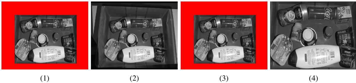
(1) Input image with reduced domain (red), (2) image for 'full_domain', (3) image for 'keep_domain', (4) image for 'crop_domain'.
