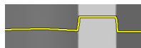
Result after sixth iteration: The edges of the right bar are restored completely.
