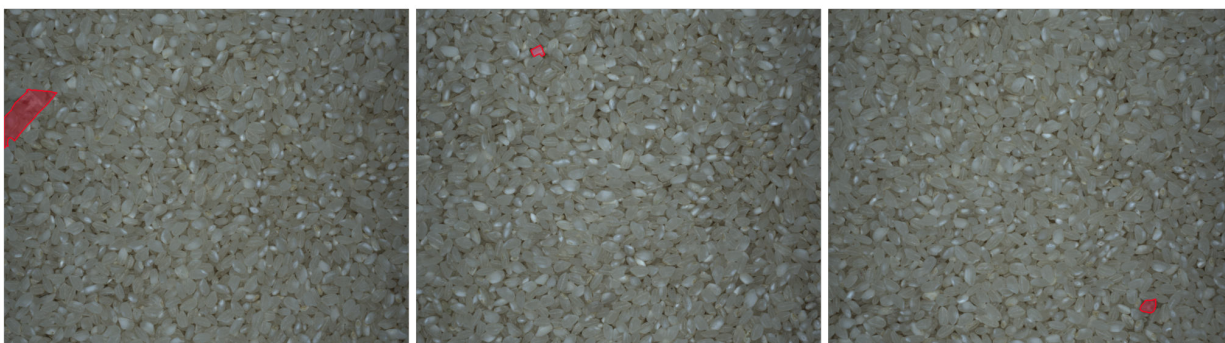
Fig. 12. Example images from the TEST_{pub} set for Rice . The defects depicted here are plastic foil and foreign bodies that were chosen to be visually similar to rice in shape, size, and color. Other defects include hairs. Defects occur all over the image, including close to the image borders.
